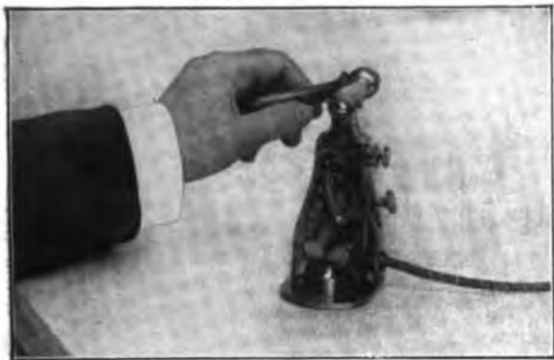
KEY IN POSITION FOR LEFT-HAND TRANSMISSION.
